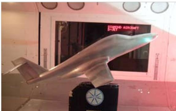
*The solid aluminum 1/5 scale instrumented D-JET wind tunnel model has made over 600 "flights" in over 100 configurations in the span of just 4 weeks. This work minimizes actual flight test time and allows a compressed flight test schedule.*
