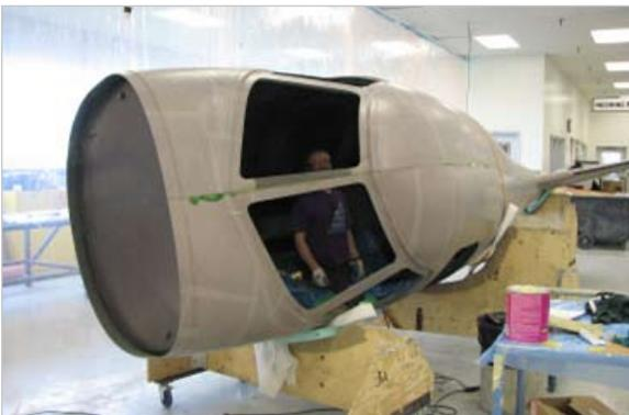
After both half-shells are cured, the internal structure is bonded into one of them and then the entire assembly is bonded together to create the rough finished fuselage, ready for trimming, secondary bonding, external finishing and final assembly.
