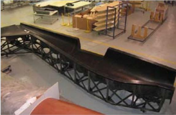
A fuselage half-shell mold is made from the master. It is made of carbon fiber reinforced epoxy such that it will expand and contract in unison with the actual part during the high temperature curing process.
