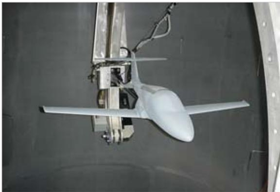
*The 1/11th scale D-JET scale model in the Spin Tunnel is "spun" at various attitudes, rotational speeds and configurations to establish the natural spin modes and speeds. This work greatly minimizes flight test risk as well as compressing development and flight test time.*
