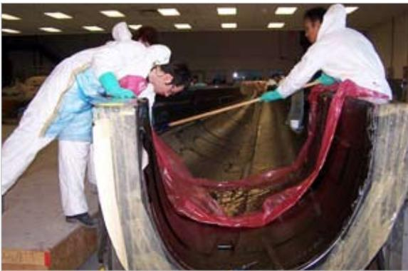
During the laminating process, successive layers of epoxy resin impregnated carbon fiber cloth are laid into the mold in strict adherence to engineering drawing. Fiber direction and positioning are critical to achieving an optimized structure.
