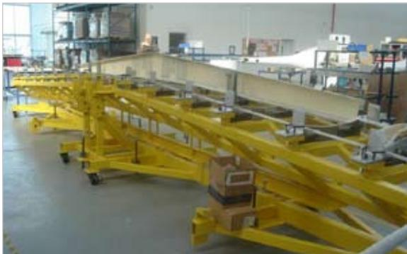
*Fixturing the main Spar is the first step in the wing structure assembly.*
