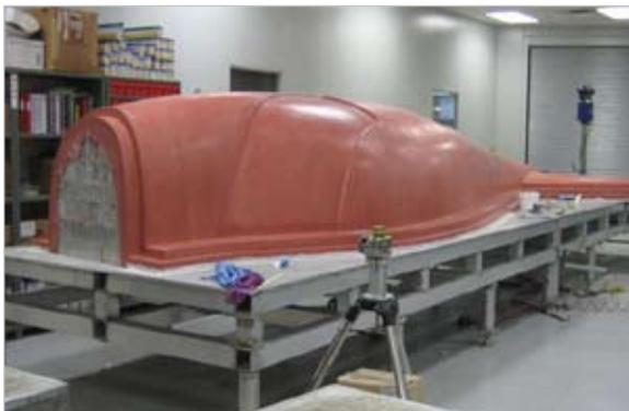
The Fuselage contour data is fed directly to a huge milling machine that machines a full scale fuselage master that exactly conforms to the intended design. This is the CAM, or Computer Aided Manufacturing part of CAD/CAM.
