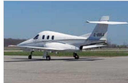
*D-JET S/N 001 taxiing out to test the new ventral strakes, which will be part of the production configuration.*
